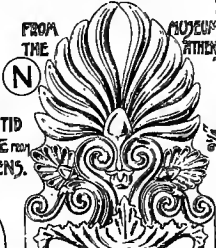
N ANTÆKA ORNAMENT TO COVER JOINT OF TILES ALONG EAVES OF ROOF
